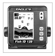
pears on the screen when you hold the PWR key down for more than a couple of seconds. When the countdown reaches zero, the unit shuts off. This prevents you from accidentally turning the unit off.
